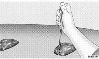
2. Rotate the socket ¼ turn and pull it from the light assembly.
